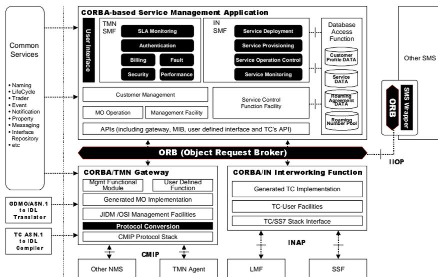
Figure 3: Platform architecture for the CORBA-based integrated control and service management system
