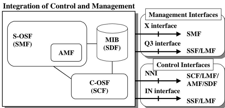
Figure 2: Integration model of service control and management functions
