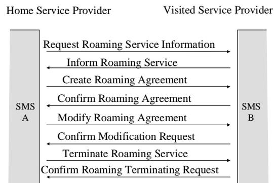
Figure 5: Management operation procedure for automatic establishment of global roaming agreement
