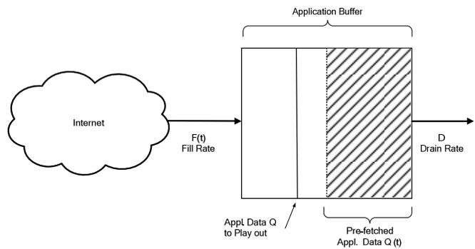
Figure 1. Application buffer structure for multimedia streaming service
