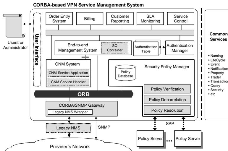
**Figure 8:** Architecture of CORBA-based VPN service management system
