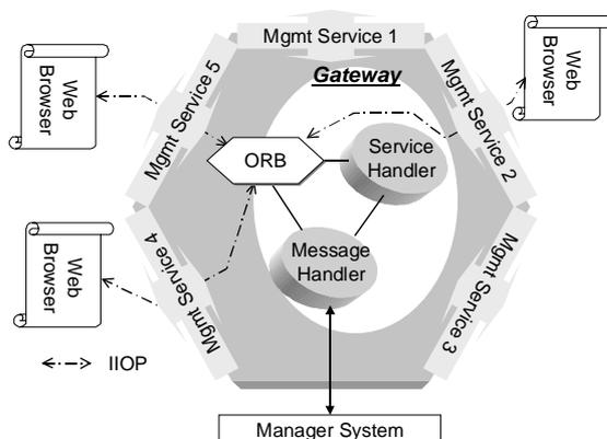
Figure 4. Architecture of Gateway
