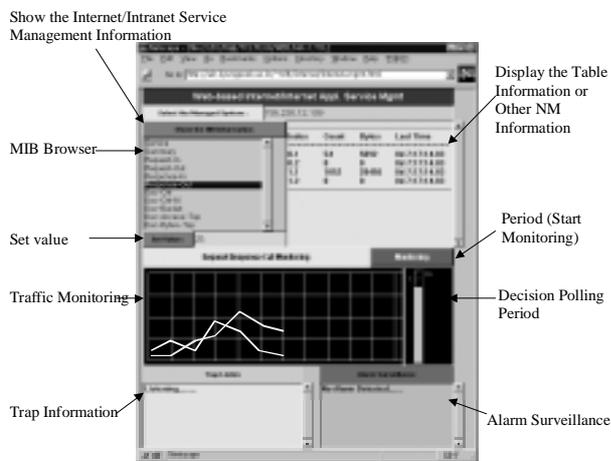
Figure 8. Implementation of Management System for Web Server
