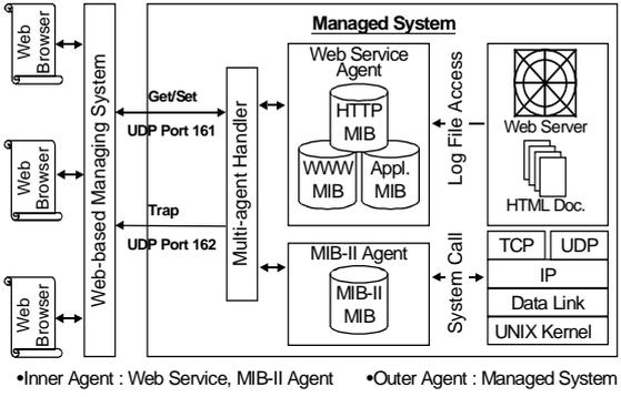
Figure 7. Architecture of Managed System
