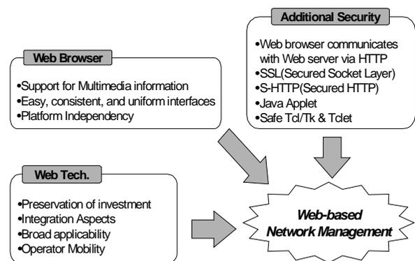
Figure 1. Advantage of Web-based Network Management System
