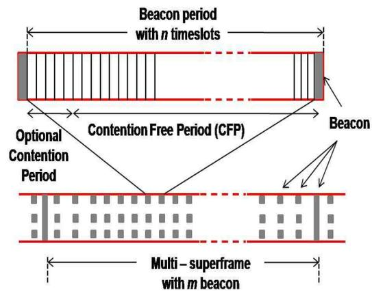
Figure 1. Super frame structure of MedMAC protocol [25]
