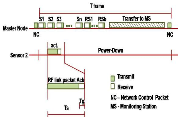
Figure 2. TDMA timing diagram [26]
