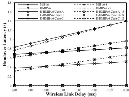
Fig 2. Impact of Wireless link delay on handover latency.
