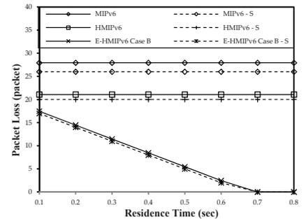
Fig 4. Packet loss as a function of residence time.
