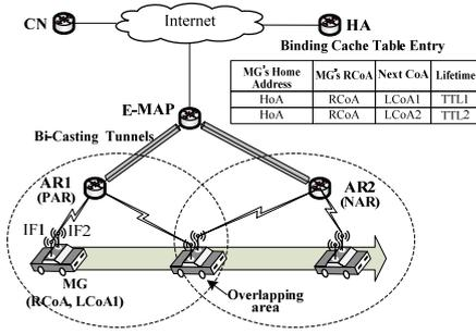
Fig. 1. Architecture of extension of HMIPv6 and mobility model using multiple tunnels.
