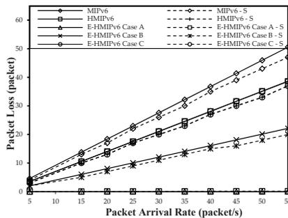
Fig 3. Packet loss as a function of packet arrival rate.
